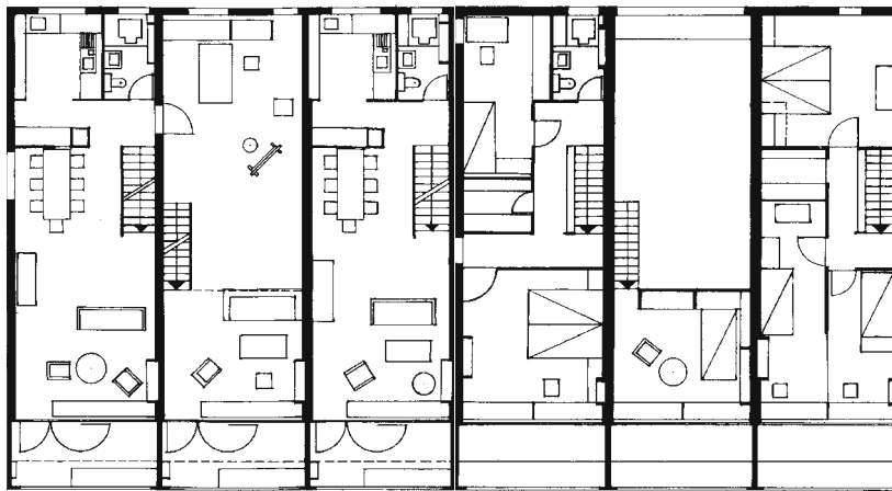
Fig. 107: Shear walls form the party walls between the maisonettes (left: main floor; right: upper floor) Atelier 5: Flamatt 1 residential development, Bern (CH), 1957–58
