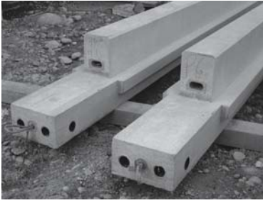
Fig. 218: Lesenes Precast concrete element Lesene (pilaster strip) in this sense is a pier-type projecting strip of wall without a capital or a base.
