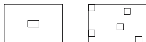
Fig. 7: Grouping versus decentralisation Schemes with stove and bathroom combined in the centre of the house (left: short service lines), and a decentralised layout (right: many service lines)
