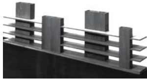
Fig. 266: Model of concrete cores Corridor access (fire-resistant escape routes), concrete towers for stability that accommodate stairs, lifts and sanitary facilities
