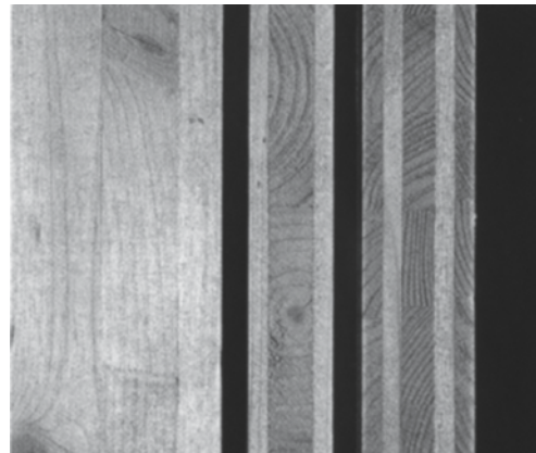
Fig. 19: Surface (sliced) and edges of 3- and 5-ply core plywood In contrast to peeled veneers, the production of sliced veneers involves cutting the trunk into thin sheets.
